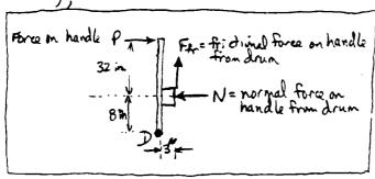
since all forces on the brake handle are balance and the hundle is stationary the handle of the breke is in static equilibrium. Therefore, the sum of the moments about point D = 0: (EMD=0)
