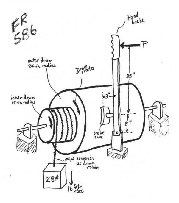
In the above diagram, the 28-1b, weight is moving downward at a velocity of 16 ft/sec. The total mass moment of inertia of the composite drum is 12 lb,-ft-sec<sup>2</sup>, and it rotates on essentially frictionless bearings. If the coefficient of friction ( $\mu$ ) between the brake and the drum is 0.40, what force (P) on the brake handle is required to stop the system in exactly two seconds?
